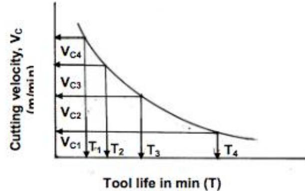
Fig. 3.2.4 Cutting velocity – tool life relationship
